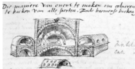
Fig. 4 Antwerpen, Museum Plantin-Moretus, Ms. n° . 64, f° 33 : Drawing of a kiln to fire stained glass in a manuscript ; ca. 1525.
