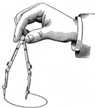
Fig. 6. Method of drawing a circle with a pair of compasses. Drawing from International Correspondence Schools, A textbook on ornamental design , Scranton, International Textbook Co., 1901, p. 8. Public domain due to age
